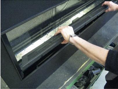
2. Remove the left and right side panels by lifting up and toward you.
