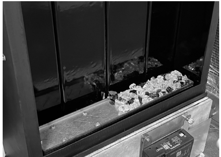
Burner Glass Media – Partially Installed
