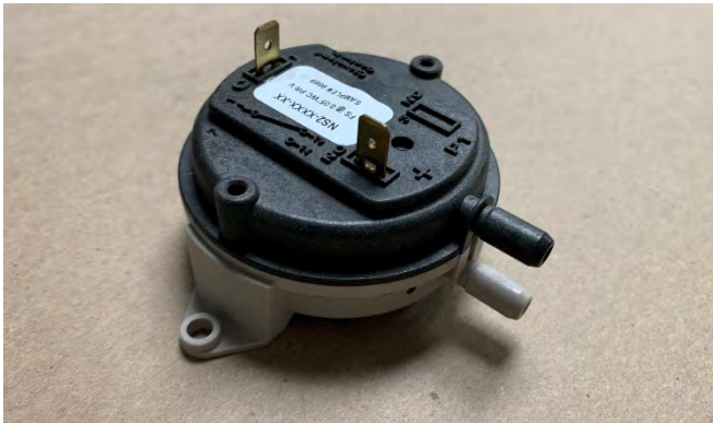
The image above shows the pressure switch ( SCPV-905PS ) used with the Self-Calibrating Power Vent. The black port should be left open to the atmosphere; the grey port should be connected to the vent pressure tap using the included silicone tubing. The pressure switch requires a negative pressure of 0.05" W.C. to confirm the power vent is running and permit the gas solenoid to open allowing the main burner to ignite.
